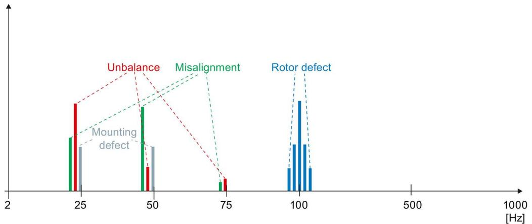
Figure 4-3 Overall spectrum of vibration velocity
