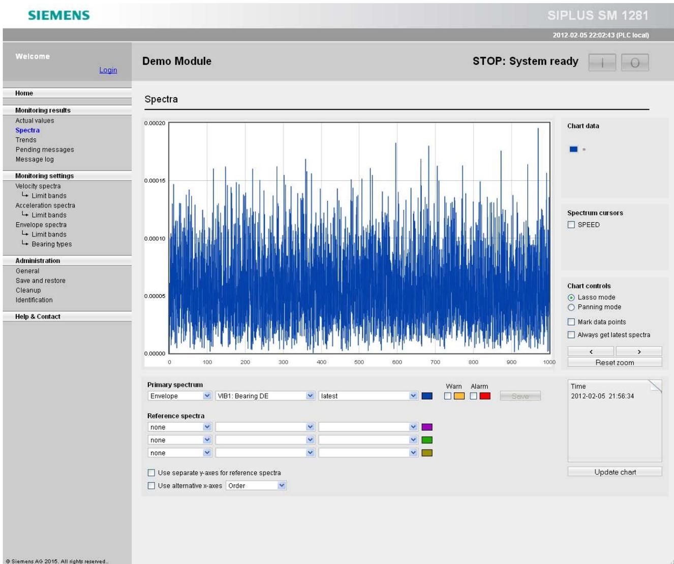
In the figure, the x axis shows the frequency and the y axis shows the amplitude. Alternatively, you can also set a scaling in "Revolutions per minute" or a non-unit "Order" (quotient of frequency and speed) for the x axis.
