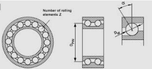
For entry of the bearing geometry, four geometric characteristic values are specified:
