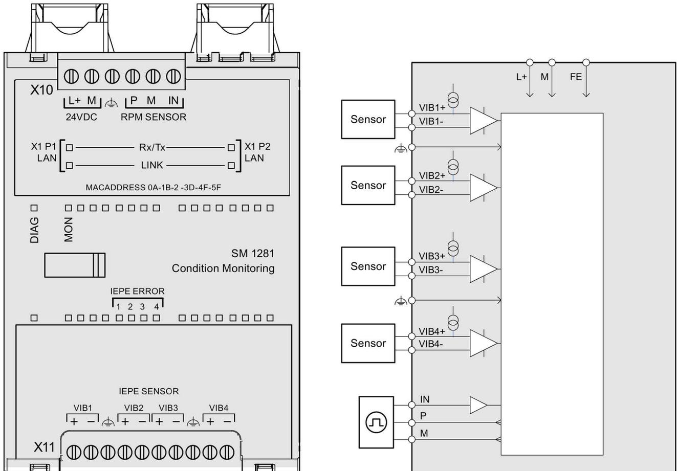
Figure 9-1 Connection diagram and block diagram
