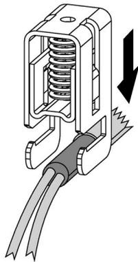
9.3 Attaching the cable shield
