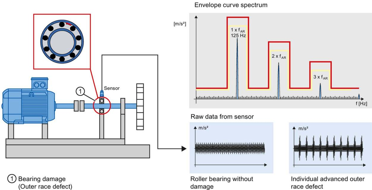
Figure 4-7 Example of envelope curve analysis
