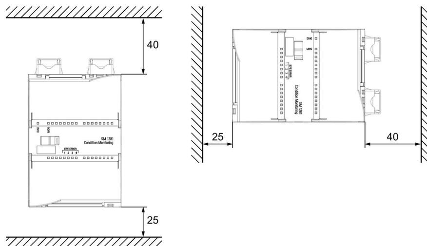
Figure 7-1 Minimum clearances with horizontal and vertical installation
