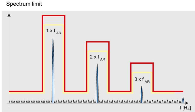
Figure 4-8 Spectrum limit band, speed-dependent
