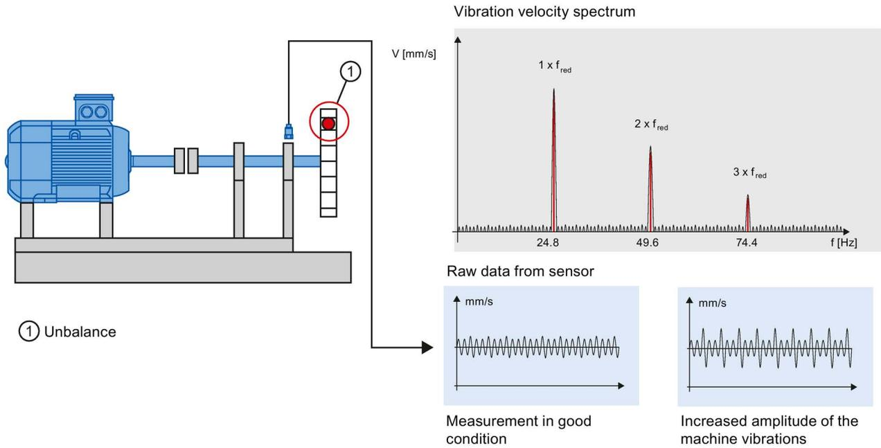
Figure 4-4 Example of a spectrum of vibration velocity (unbalance)
