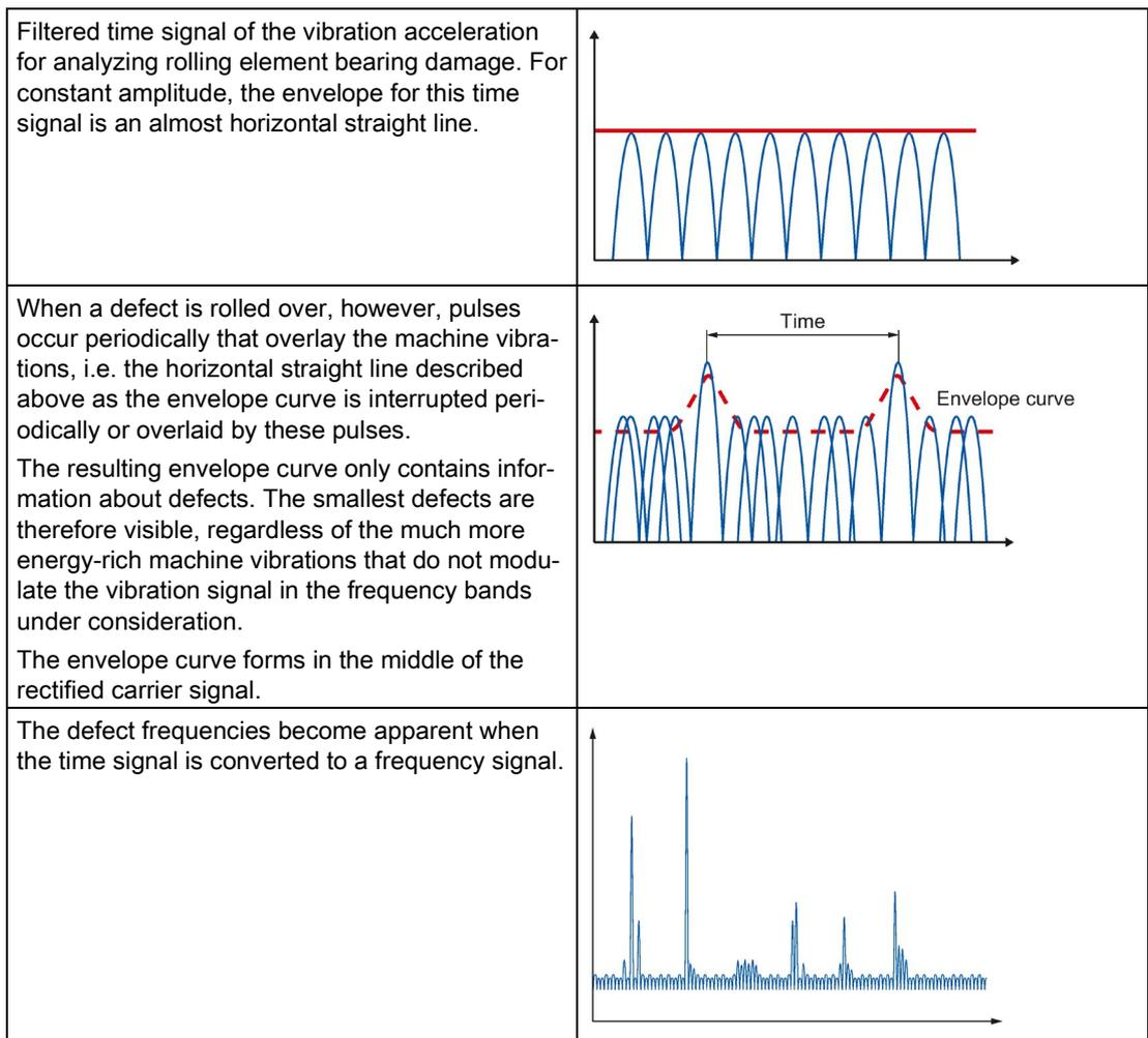
4.6.4.2 Application example bearing analysis: Rolling element bearing damage (envelope curve)
