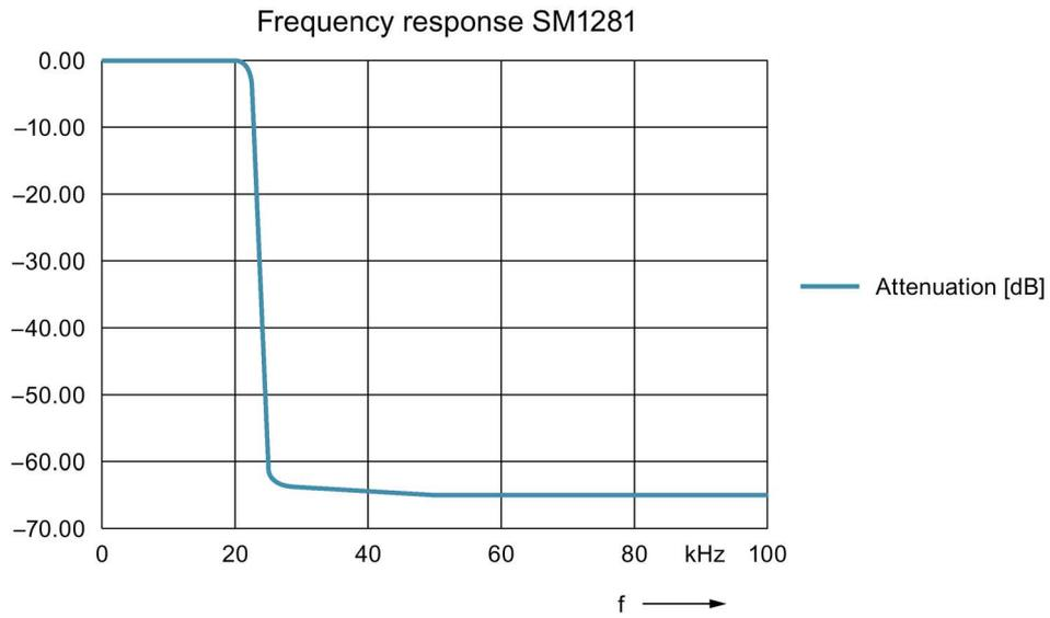
Figure 15-1 Filter characteristic curve analog inputs SM1281
