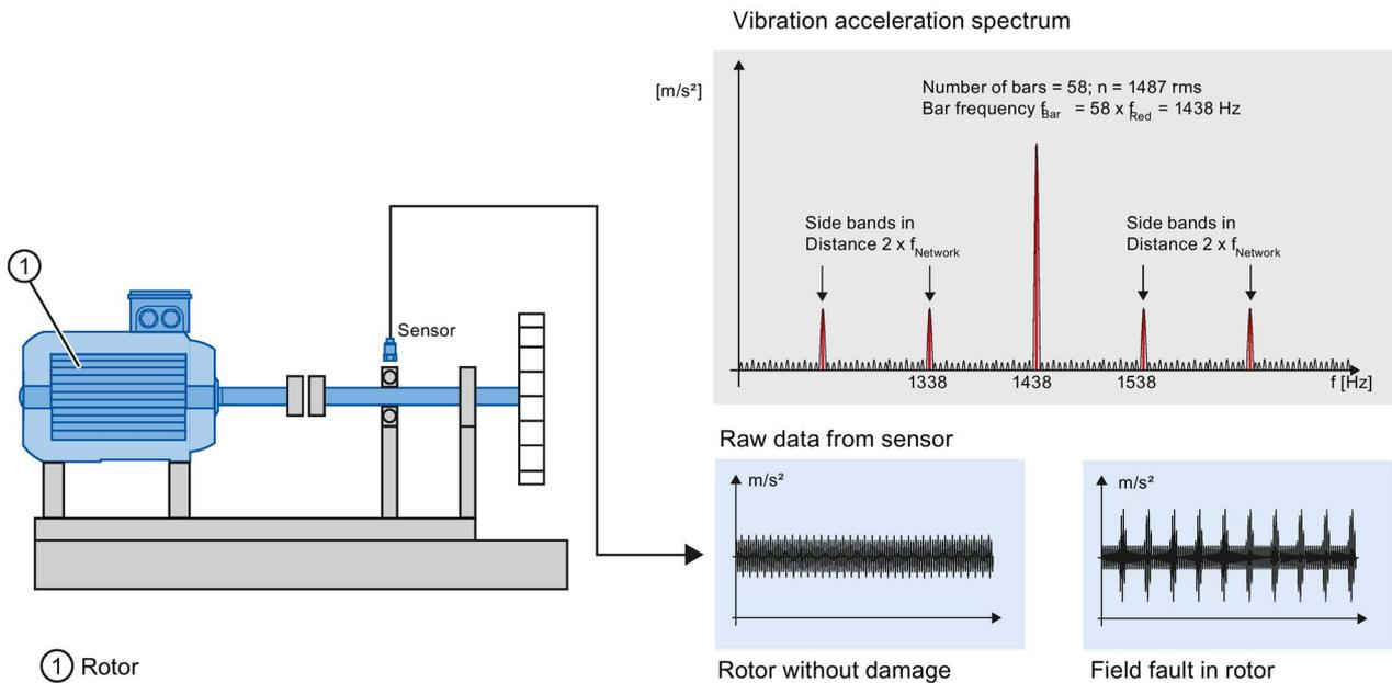
Figure 4-6 Example: Spectrum of the vibration acceleration (rotor field fault)
