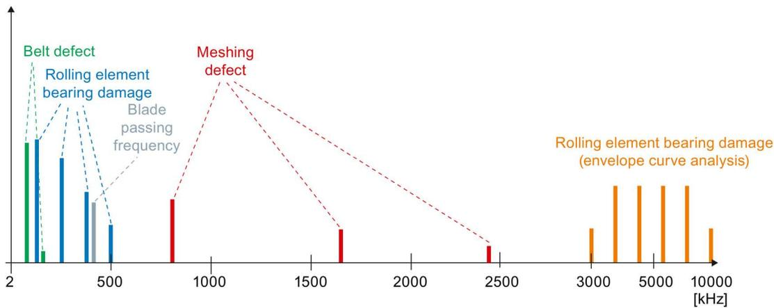
Figure 4-5 Overall spectrum of vibration acceleration
