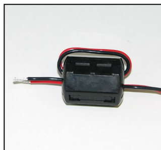
Figure 2-7 EMI Filter Installed
