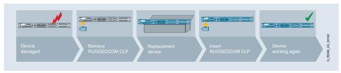
The CLP interface allows for quick and easy exchange of defective devices in the field.
