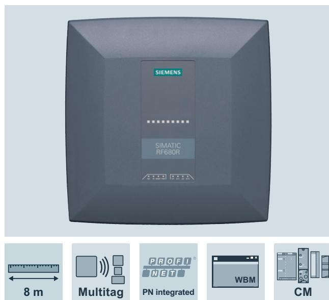
The high-performance SIMATIC RF680R reader has four antenna connections that can be configured as required for individual read stations, or as gates. The high radiated power of up to 2 W ERP / 4 W EIRP (dependent on antenna and cable) permits long ranges of up to 8 m in portal applications.
