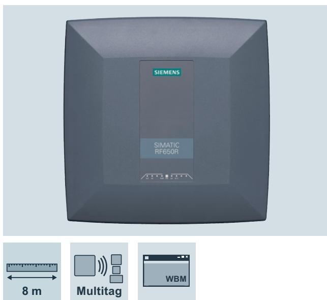
The high-performance SIMATIC RF650R reader has four antenna connections that can be configured as required for individual read stations, or as gates. The high radiated power of up to 2 W ERP / 4 W EIRP (dependent on antenna and cable) permits long ranges of up to 8 m in portal applications.
