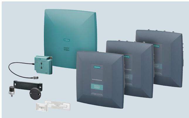
Identification tasks in the UHF range (865 to 868 MHz, 902 to 928 MHz, and 920 to 925 MHz) that demand a wide range of several meters are implemented with SIMATIC RF600. The system is suitable for storing and recording a unique identification according to the EPCglobal standard (Electronic Product Code) on products, containers or transport units. Storage of additional, freely-definable user data is also possible.
