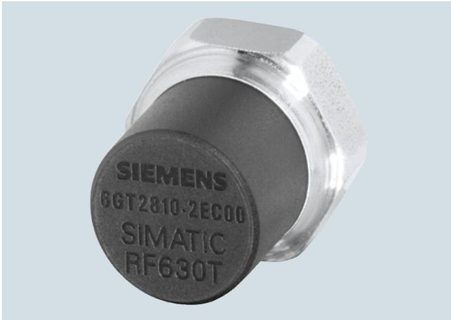
The SIMATIC RF630T screw transponder is particularly suitable for controlling and monitoring production processes. It can be automatically screwed on to products such as motors or gearbox casings by means of robots and using the M6 grub screw.
