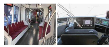
speeds up to 55 mph, carrying close to 185 passengers in each vehicle with the ability to operate in multiple vehicle consists (up to four). These light rail vehicles remove automobiles off the road, in turn helping cities decrease their CO2 emissions.
