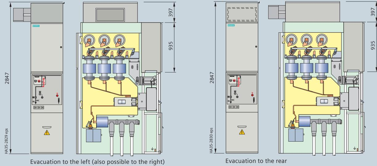
**NXPLUS DBB with horizontal pressure relief duct and evacuation**
