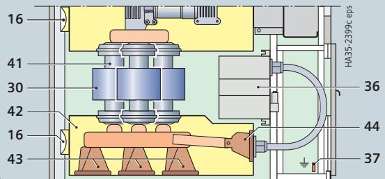
Panel with separate inside cone up to 40.5 kV
