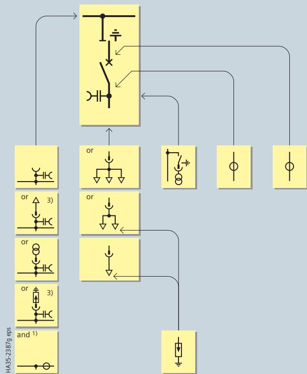
**Circuit-breaker panel (cable connection as inside cone)**
