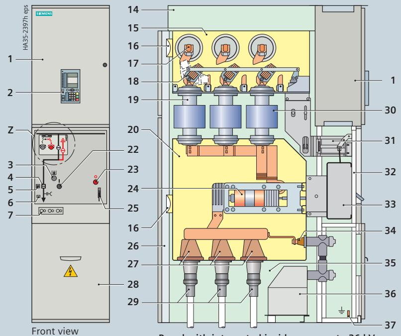
Panel with integrated inside cone up to 36 kV
