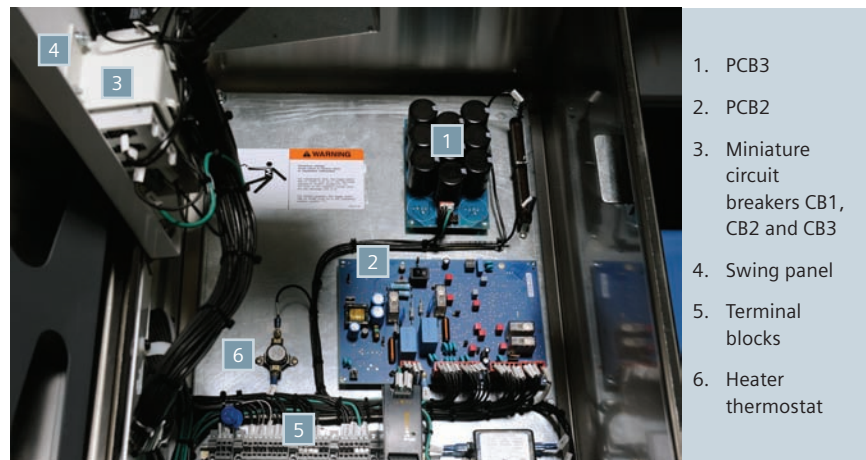
Figure 11: Three-phase type SDR controller with swing panel open
