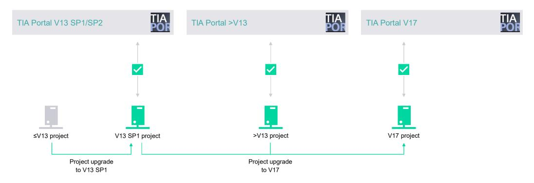
Side-by-side installation of V13 SP1/SP2 up to V17 allows access to all project versions. The V17 license can be used for all available versions from V11.
