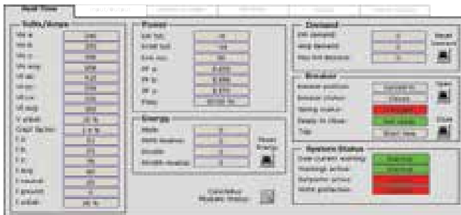
Real-time data from WL breakers with remote open/close capability
