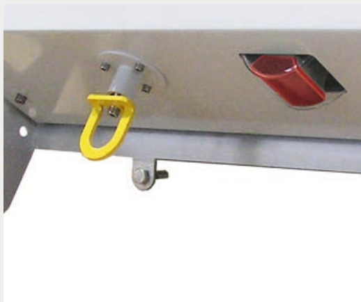
Lockout handle – pushed in (operational position)
