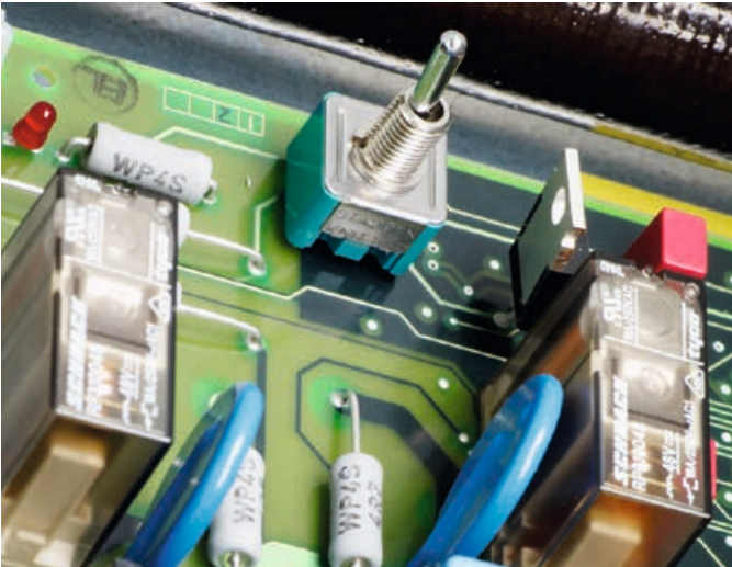
Switch unit driver – discharge switch for the capacitor
