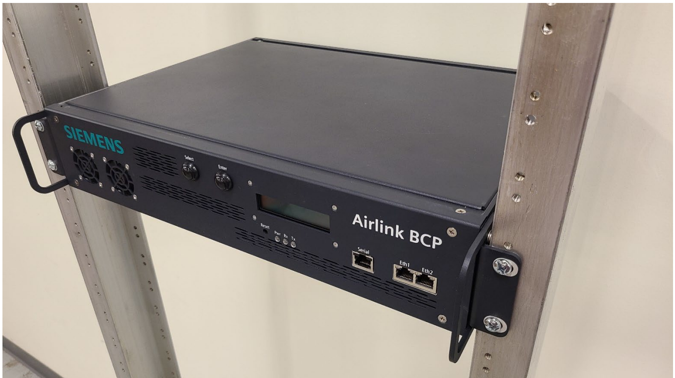
Figure 4-2 Airlink BCP Top/Front View when Mounted to Rack
