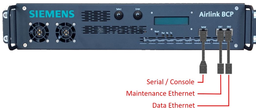
Figure 4-9 Airlink BCP Typical Interconnect Diagram – Front View
