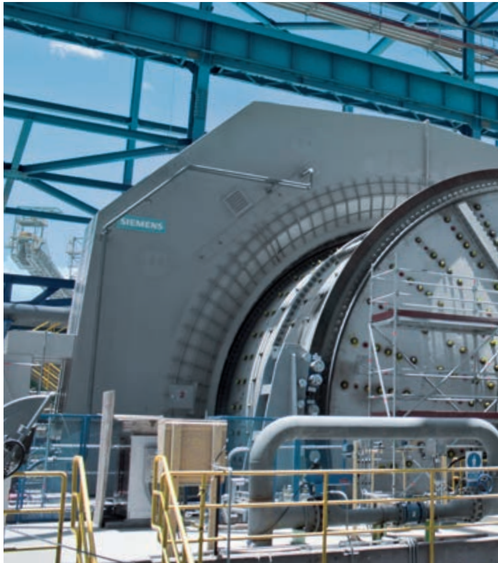
Antapaccay's 40ft SAG Mill with a 24MW gearless drive from Siemens
