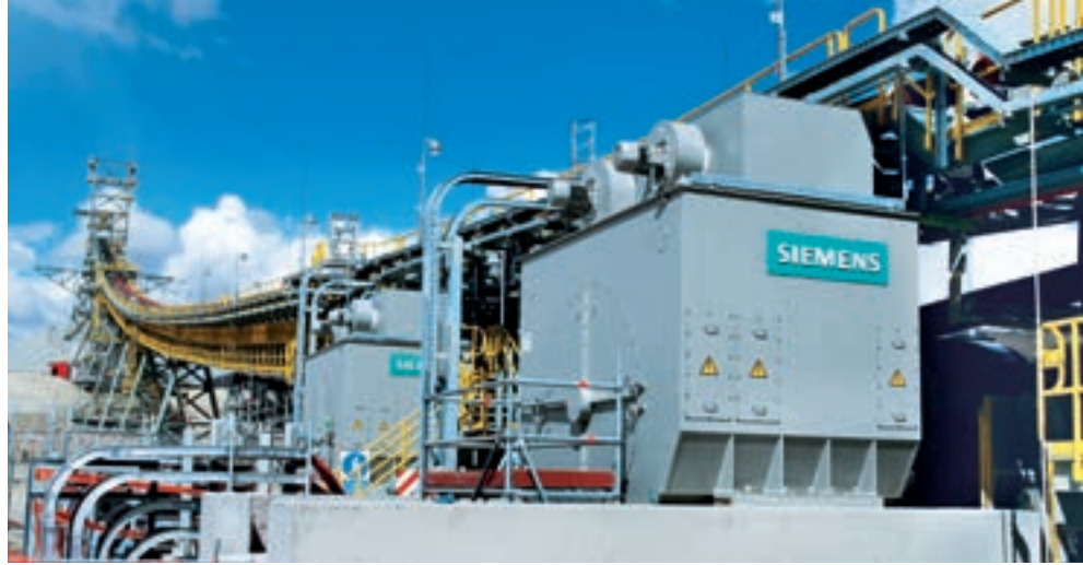
The drive station of the 6.5 km belt conveyor at the tail of the conveyor toward the stockpile
