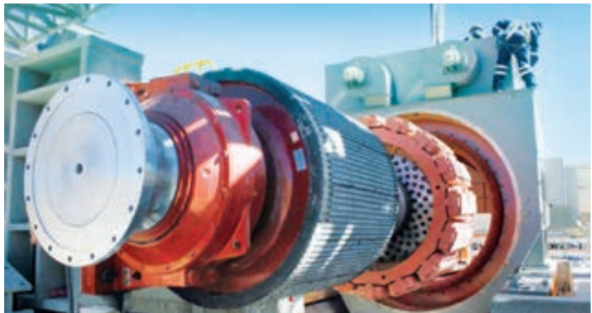
Drive pulley with the rotor attached on the same shaft and the stator shifted back into maintenance position (picture taken during installation)
