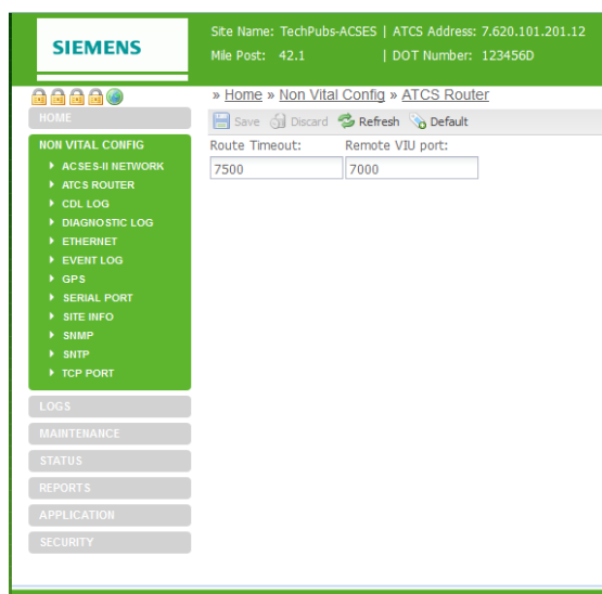
Figure 7-20 ATCS Router Configuration Screen
