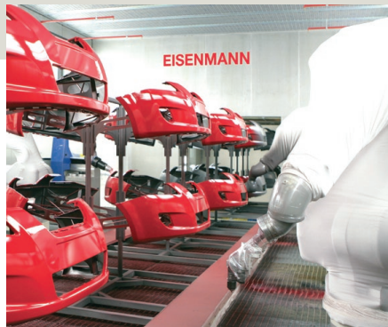
Automotive subassembly paint line delivered by Eisenmann.
