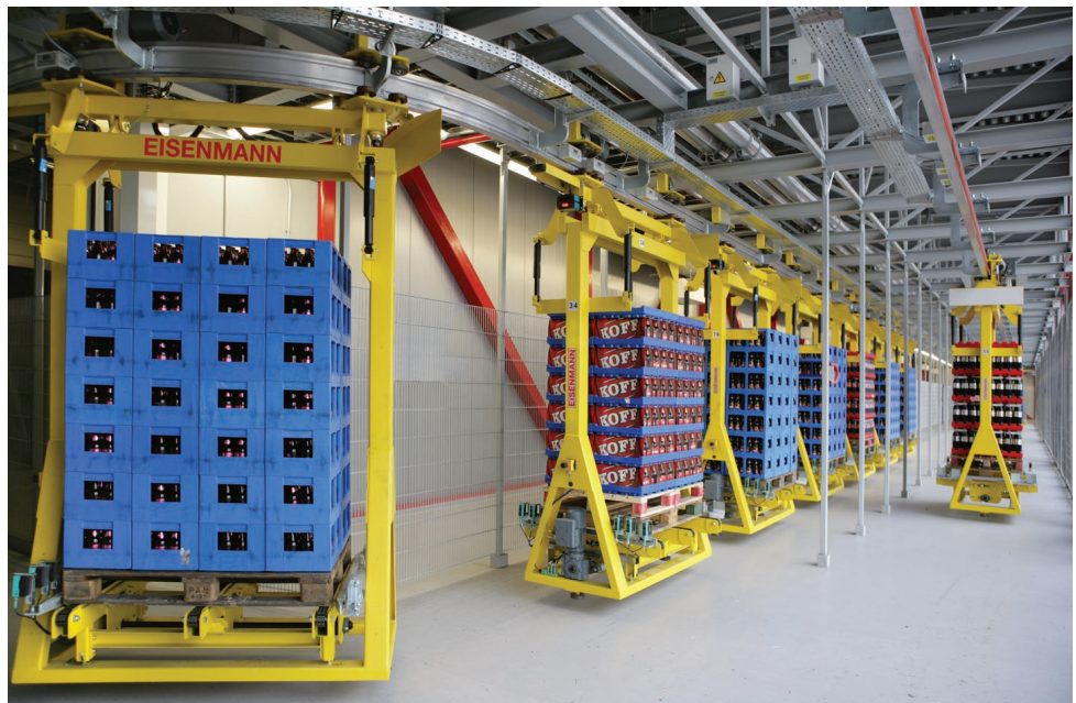
Eisenmann electrified monorail system.
