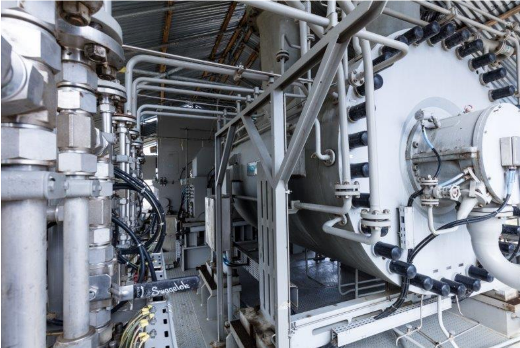
Above: A typical single-shaft, vertically-split Siemens STC-SV turbocompressor used for LNG service.
