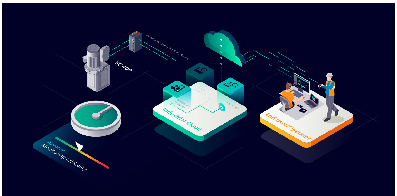
System overview of the condition monitoring of an aerator used at a wastewater treatment plant of Scottish Water.
