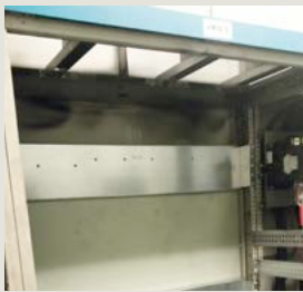
1. Install SINAMICS chassis supporting mechanics
