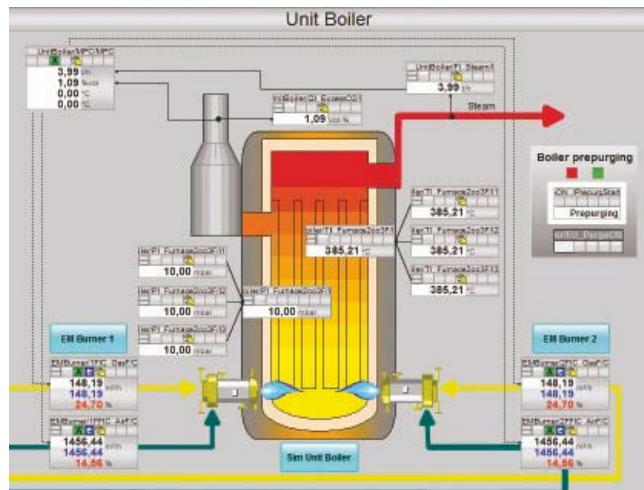
Process screen from a Burner Management System (BMS)
