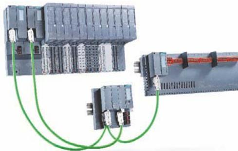
The switch with dual network access functionality (DNA or Y-switch functionality) connects a redundant PROFINET ring consisting of S2 devices (field area) to a high-availability PROFINET system (R1 system). Besides the two "Y-switch" ports, two other switch ports are also available at the device end. These can for example be used to operate an MRP ring.
