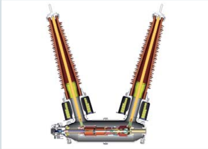
Figure 3: One pole of a dead tank circuit breaker
