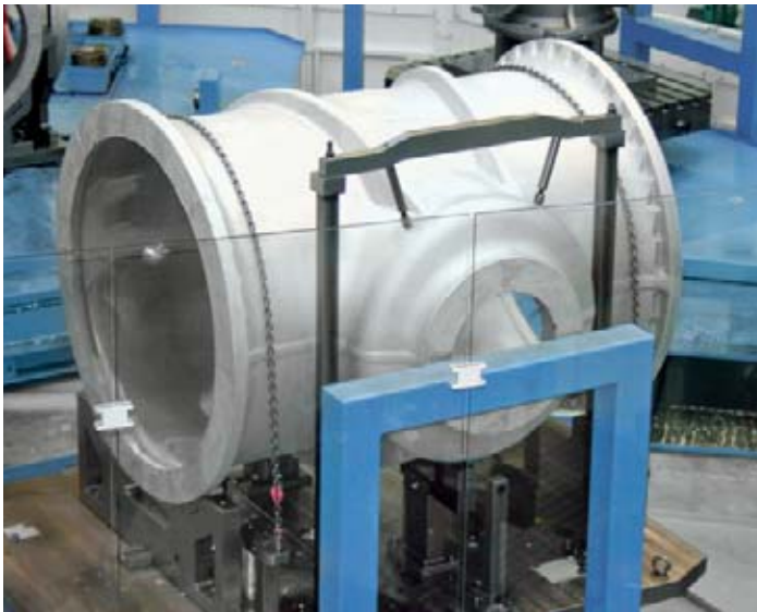
Figure 1: Unfinished casting housing in a machining centre
