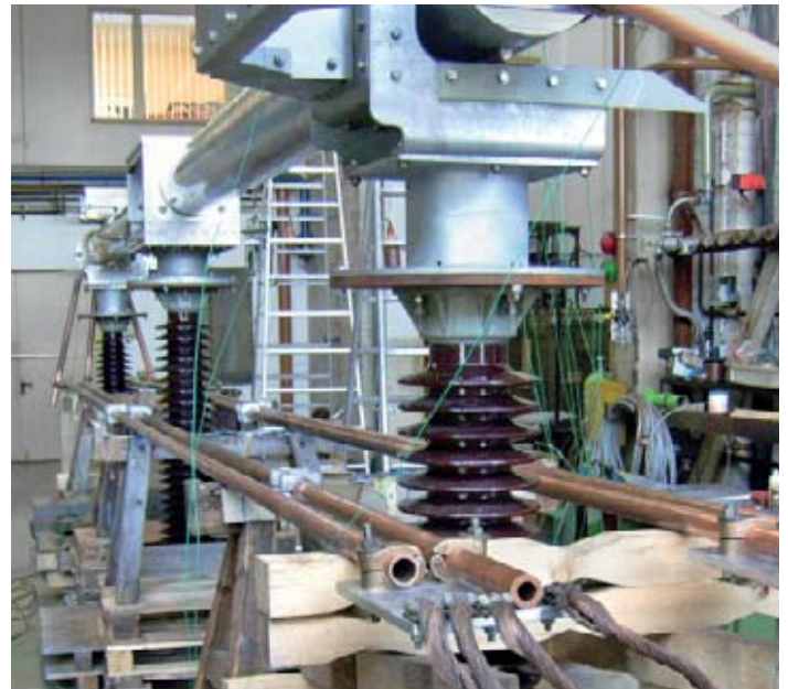
Figure 6: Setup for temperature rise test
