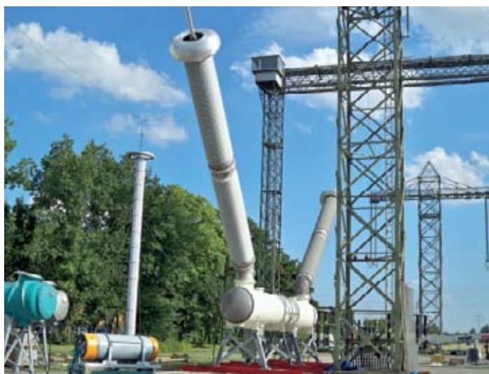
Figure 7: Test setup of Siemens 8DQ1-P5-1100 kV – 50 kA during dielectric test at FGH
