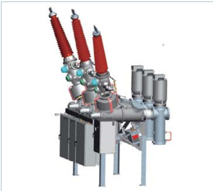
Figure 9: Assembly with cable connection and VT
