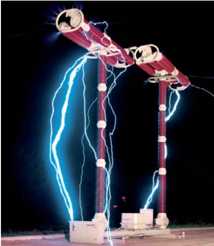
Figure 4: High Voltage Test at a 800 kV Life Tank Breaker
