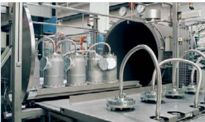
Figure 6: Test system for cumulative leakage measurements
