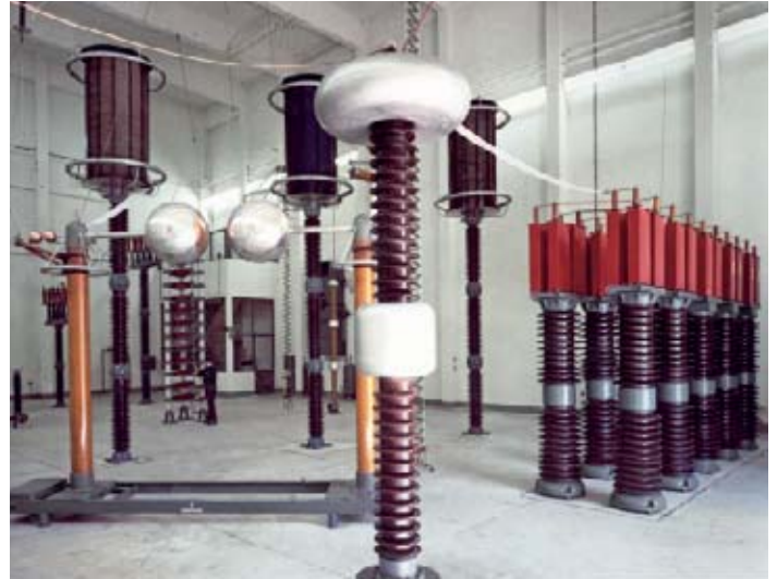
Figure 1: Configuration of the first synthetic circuit from 1962 in the switching test facility
