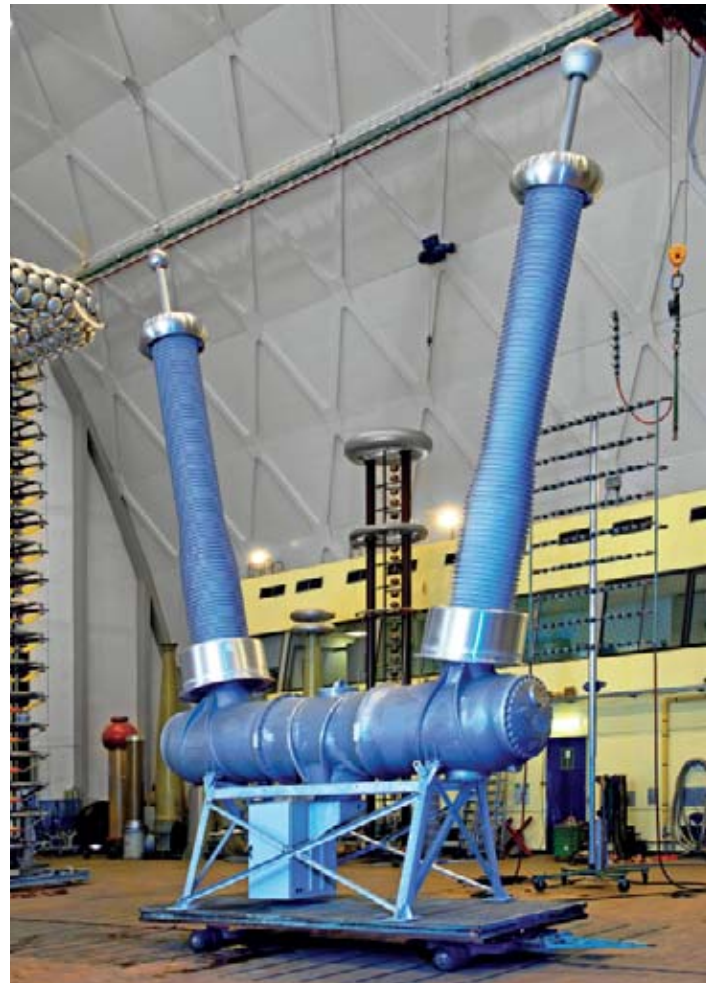
Figure 4: 500 kV Dead tank circuit breaker for 63 kA
