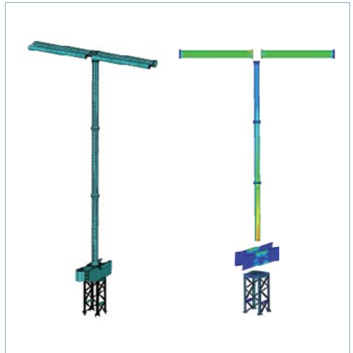
Figure 10: Geometry of FEM-Model (left) and calculated mechanical stresses (right)
