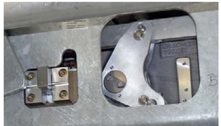
Figure 6: Blocking system and corner gear lever in the base frame of the 145 kV DCB
