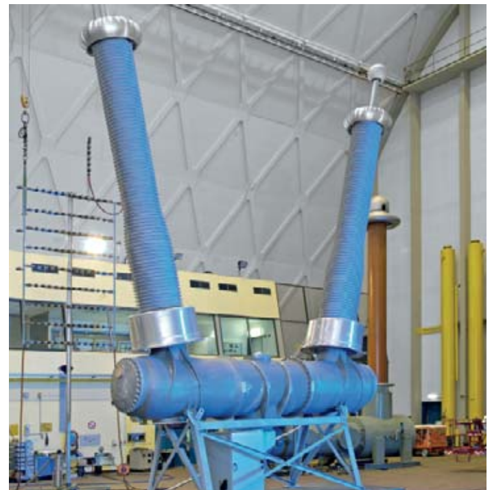
b.: ring core current transformer on the bushings of a dead tank breaker
