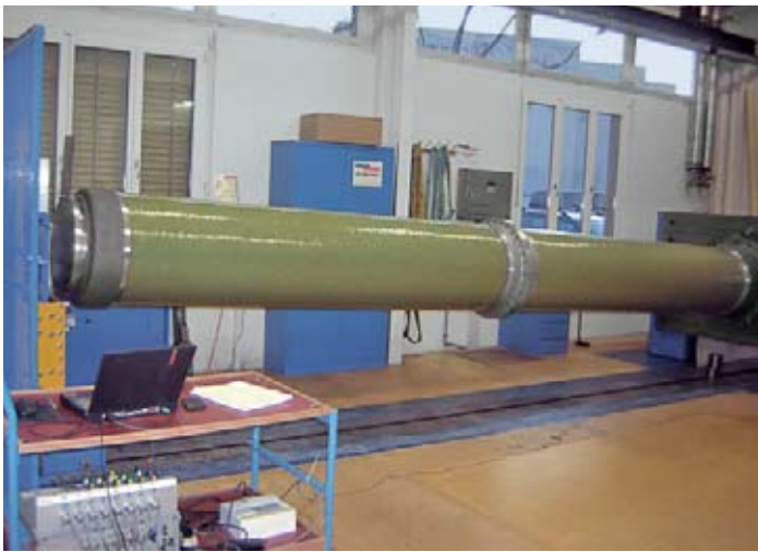
Figure 2: Setup for cantilever bending tests
