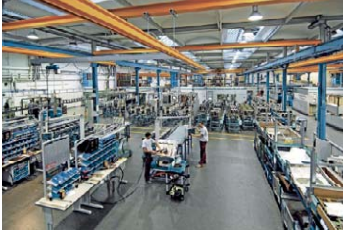
Figure 11: Assembling lines for medium voltage Vacuum Breakers
