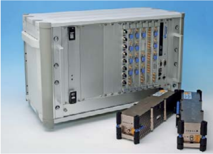
Figure 4: Each transmitter (bottom right) can be connected with any receiver rack (centre) via a fiber-optic patch panel
