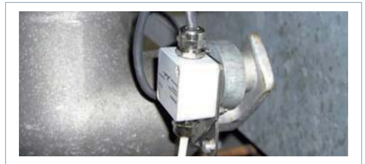
Figure 13: Reference contact at the corner gear
