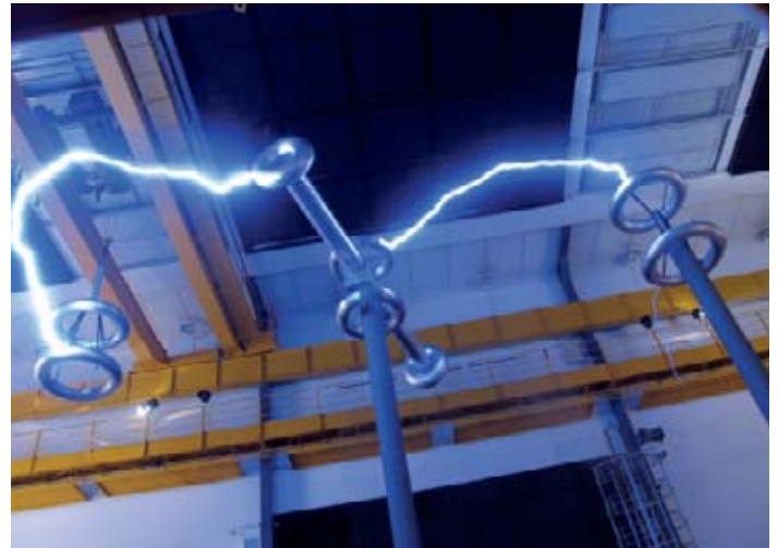
Figure 3: Preliminary study on disconnector gap with switching impulse voltage
