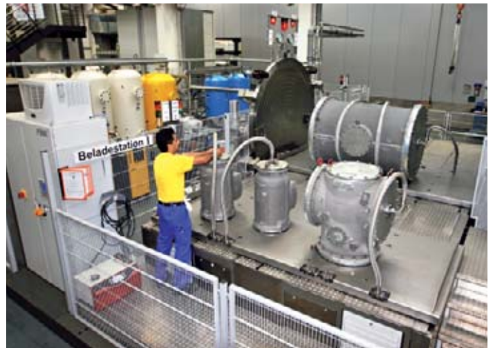
Figure 3: Connecting the test pieces to the testing system
