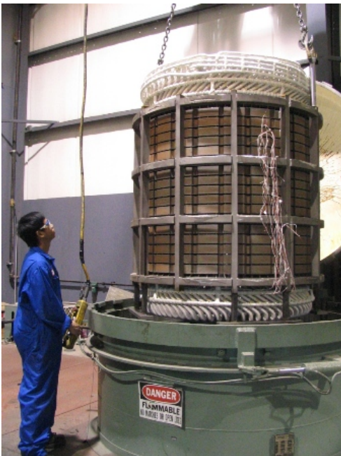
A rewind motor stator is lowered into the vacuum pressure impregnation tank during the motor refurbishment process at the Calgary TurboCare facility
