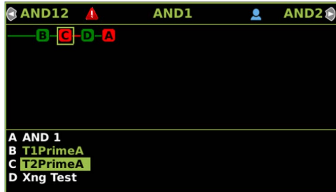
Figure 21 AND Logic Example
