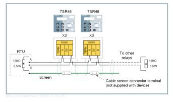
Figure 3.3/1 Typical RS485 Connection
