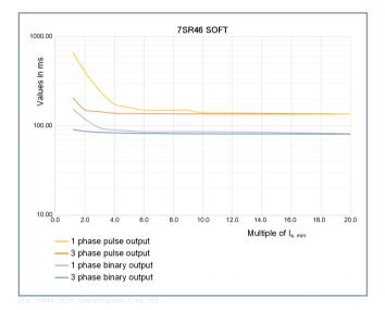
Figure 3.1/1 50LC/SOTF for 3-Phase, 1-Phase with Binary Output and Pulse Output
