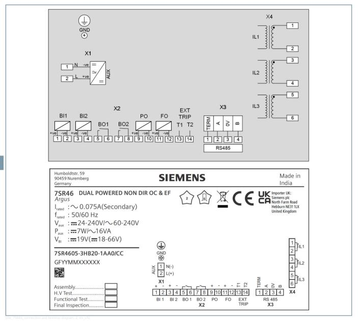
Figure 4.1/1 Connection Diagram and Terminal Label
