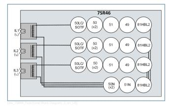
Figure 2.2/2 Functional Diagram of 7SR46 Dual-Powered Non-Directional Overcurrent and Earth Fault Relay
