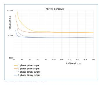
Figure 3.1/2 Operating Time for 3-phase, 1-phase with Binary Output and Pulse Output
