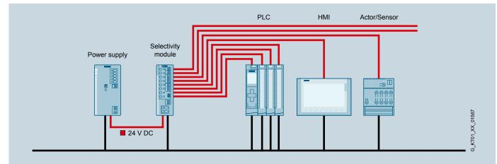
As an electronic monitor, the SITOP selectivity module switches faulty 24 V DC load circuits off immediately, and continues to supply the other loads without any interruption.
