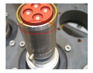
Check connector body for damage such as dents, scratches (Picture shows damage to body)
