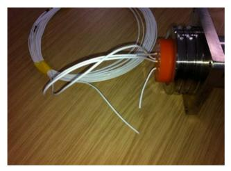
Check tail wires along their length, for damage or breaks. (Picture shows broken tail wire)
