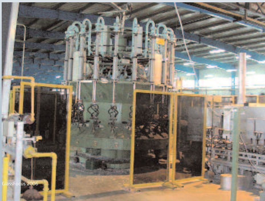
The drives for the many axes of the plant use Simodrive 611 converters
