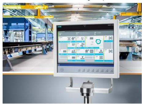
Siemens has extended its system family of all-round protected HMI (Human Machine Interface) devices for machine-related, cabinet-free visualization and automation. The all-round IP66 protected Simatic HMI Thin Client Ex OG is the new addition to the series of Ex HMI devices.
