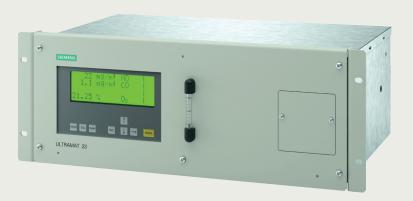
Multi-Component NDIR Gas Analyzer Up to 4 gas components can be measured simultaneously including three IR active gases such as  $CH_4$ ,  $CO_2$ , CO, NO,  $SO_2$ , and in addition can measure  $O_2$  using an electrochemical cell.
