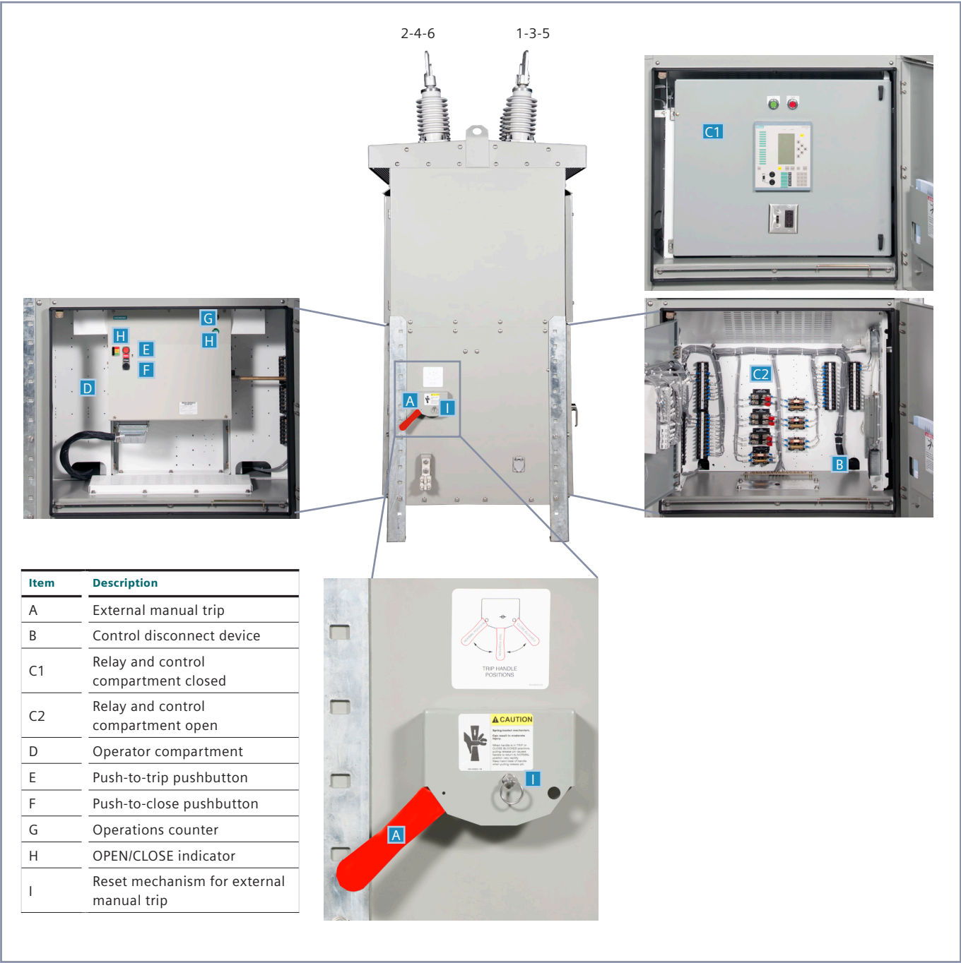
Figure 8: Relay and control and operator compartments for type SDV7-MA-AR circuit breaker with magnetic-actuator operator
