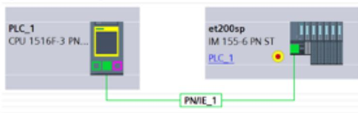
Figure 4-2 ET 200SP station configuration
