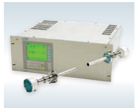
Siemens LDS6 Analyzer
