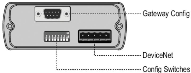
2. On the EtherNet/IP or Modbus TCP/IP side of the Anybus X Gateway connect your RS-232 DB9FF Null Modem Cable to the Gateway Config Port and the serial port on your computer.
