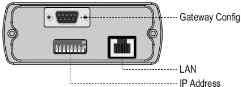
3. On the Modbus RTU side of the Anybus X Gateway connect your RS-232 DB9FF Null Modem Cable to the Gateway Config Port and the serial port on your computer.
