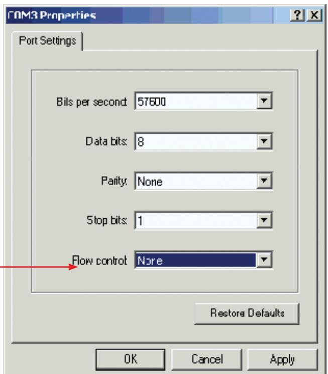
Press the CONFIGURE button to set up the communication parameters of the port to connect with the gateway
