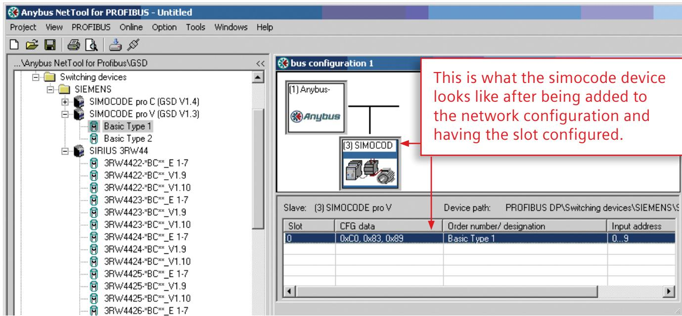
This is what the simocode device looks like after being added to the network configuration and having the slot configured.
