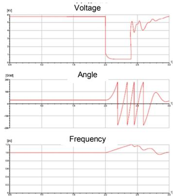
Figure 3: Determination of the de-coupling criteria with dynamic simulations
