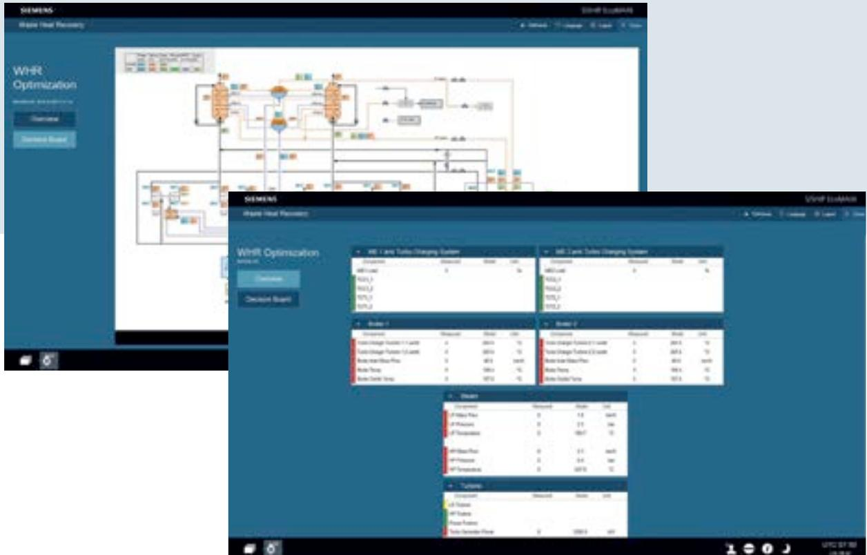
The EcoMAIN WHR system optimization application provides decision support in order to optimizing waste heat recovery from the exhaust gas of the main engine.
