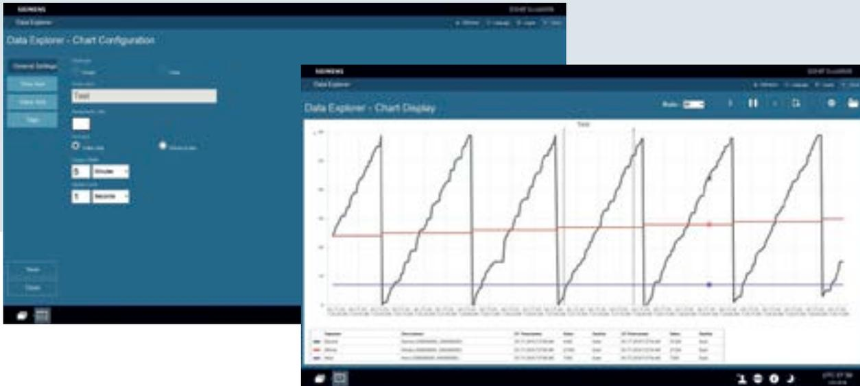
The Data Explorer tool offers easy data analysis, allowing the operator to compare data in a graphical manner. An intuitive configuration dialog box can be used to set up this data tool according to individual needs. Chart configurations can be saved in the EcoMAIN system and reopened at any time, whenever needed. Data charts can be individually created by each user and also made public to all users. Data Explorer shows actual online data as well as historical data.
