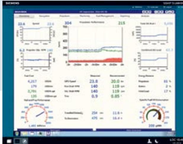
The MAREN Energy Efficiency application is powered by our partner company Marorka. MAREN fulfills a wide range of energy efficiency tasks and is integrated into the EcoMAIN system.
