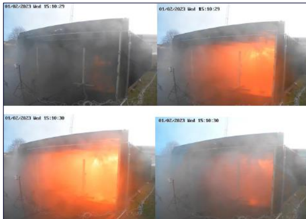
Figure 11: Various phases of Test 2, Ref. 6, showing an intense fire in the simulated garage space
