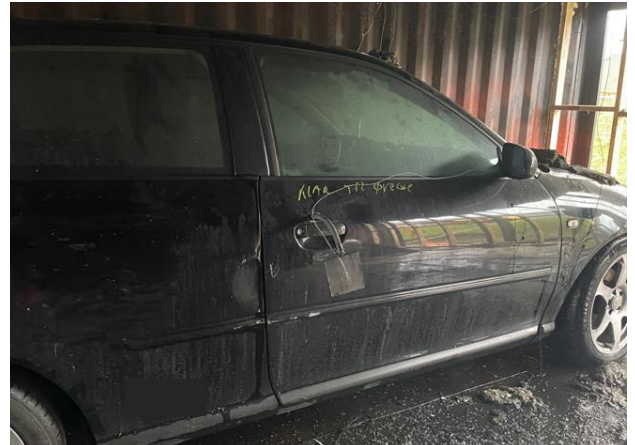
Figure 12: Car adjacent to burnt EV, showing no damage after intense fire in Test 2, Ref. 6, with high pressure water mist fire suppression
