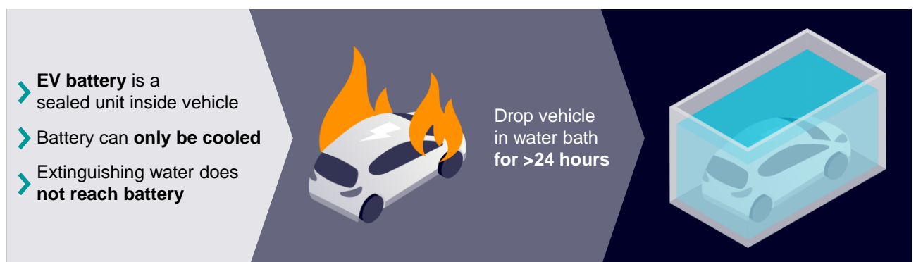
Figure 5: Water cooling of vehicles with battery fires
