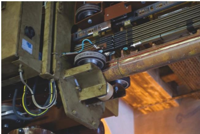
IWLan antennas provide continuous wireless communication even at segment transitions. The Rapid Roaming function provides transfer times of less than 32 milliseconds between access points.
