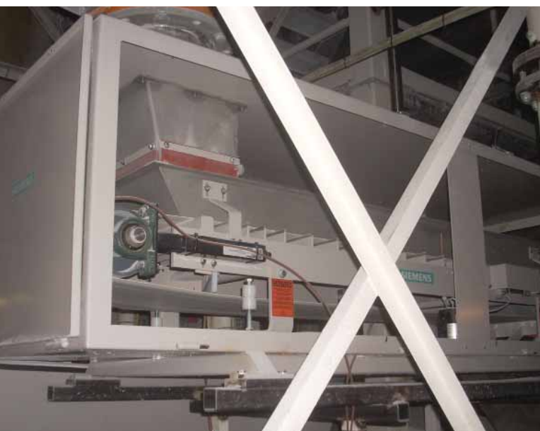
Installing and testing SITRANS WW200 was a simple process. NOPA's operators have been pleased with the weighfeeder's reduced maintenance requirements.
