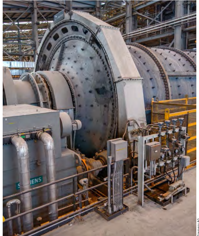
The solution for the Arizona copper concentrator features the world's largest dual-pinion drive systems with low-speed induction motors
