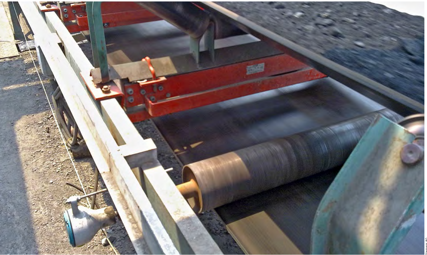
A Milltronics belt scale and speed sensor on a conveyor belt moving mining material
