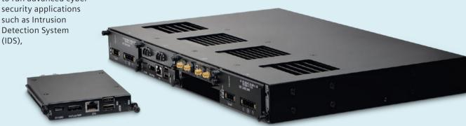
Deep Packet Inspection (DPI) and Next Generation Firewall (NGFW) from industry leaders in cybersecurity. The APE1808 can operate from -40°C to +75°C, making it suitable for mission-critical applications in industries with harsh environments, including electrical power, oil & gas, and transportation. Ruggedcom APE1808 can be inserted in devices from the RX1500 family of products and allows for
