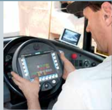
Fig. 2: Thanks to the use of Mobile Panels as seen here for the extraction of graywacke in the Treis-Karden quarry, mobile sub-systems can be integrated into the plant automation via industrial wireless networks (IWLANS)
