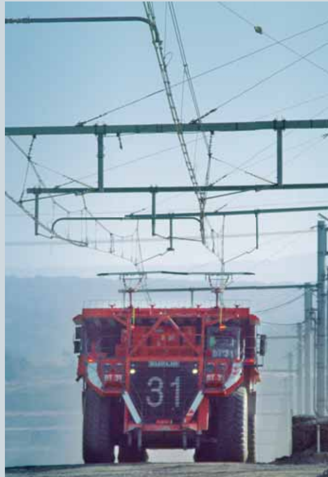
Cantenaries on the mine's gradients, similar to those used with rail travel, provide the trucks with electricity. The result: lower fuel consumption and higher speeds on ramps
