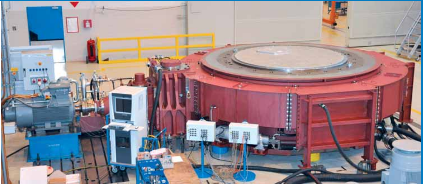
Fig. 3: Test run of the 6,600 kW mill support with a drive module
