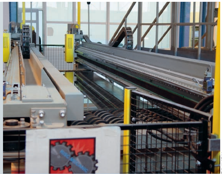
Perfect cutting with high technology: The cross-cut bridges on the I-Scan float glass line
