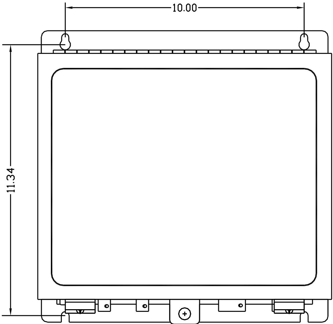
Figure 1. LFO Mounting Hole Dimensions
