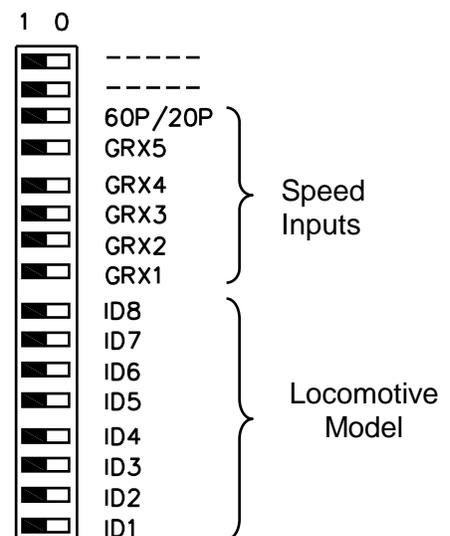
Figure 6. 16 Position DIP Switch
