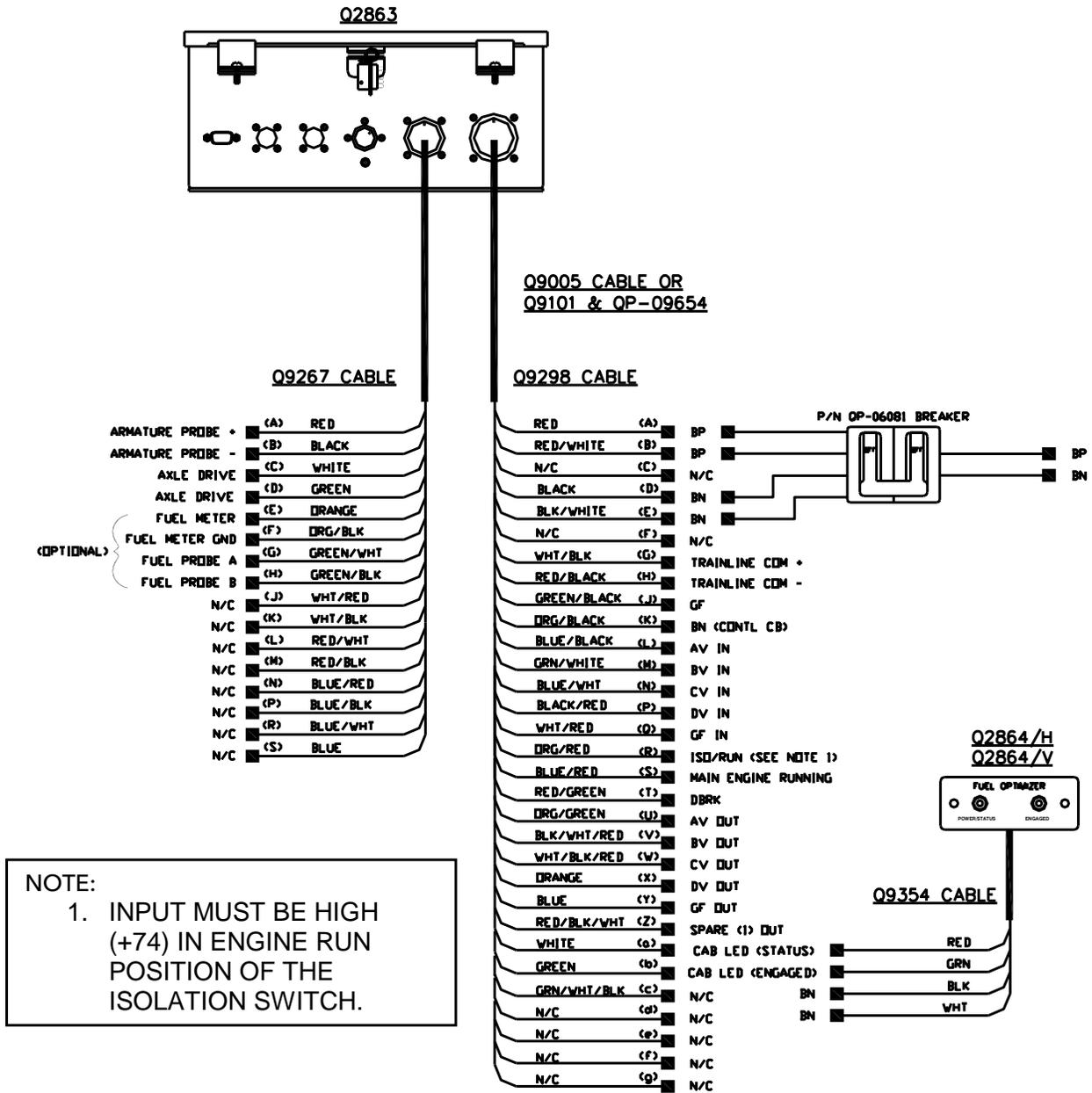
Figure 4. LFO Interface Cable Wiring Diagram
