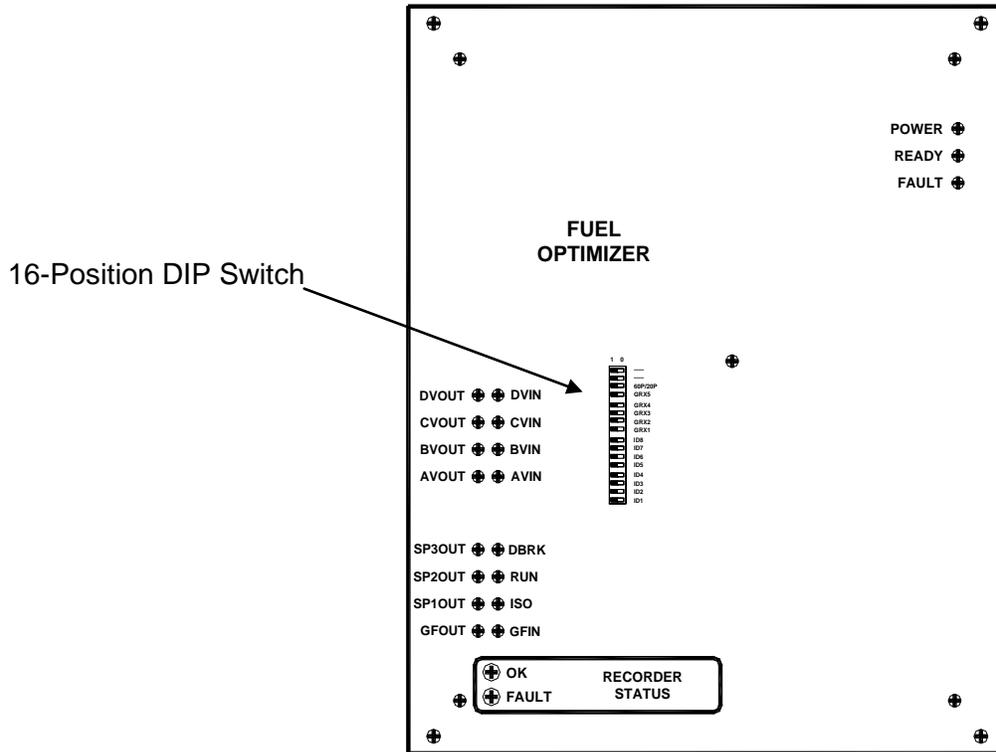
Figure 5. LFO Front Panel (Located Under Cover)
