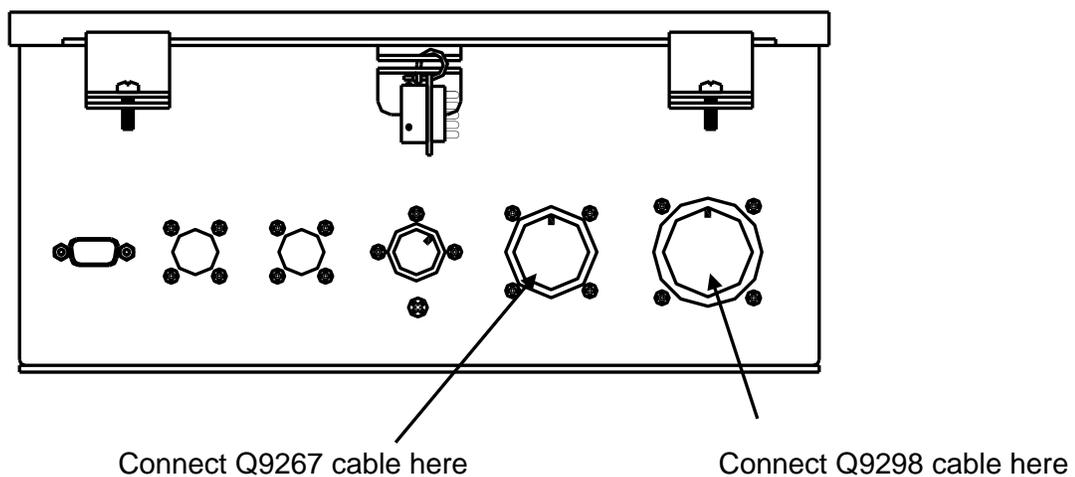
**Figure 3. LFO Cable Interface Locations**
