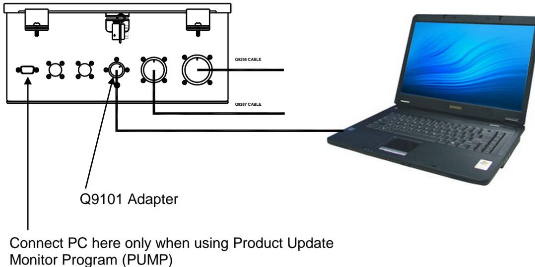
**Figure 7. Laptop Computer Connection to LFO**
