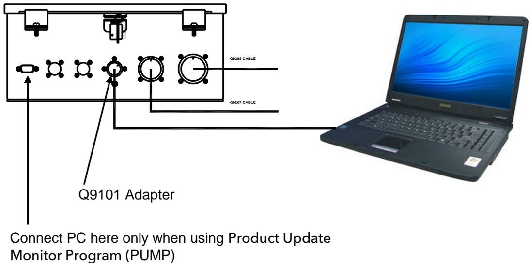
**Figure 8. Laptop Computer Connection to LFO**
