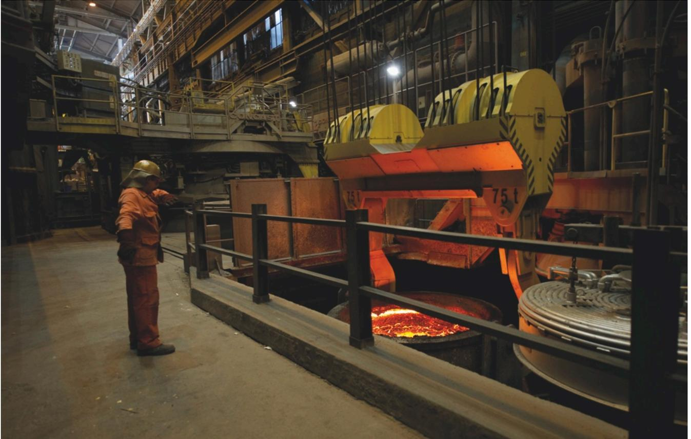
The pig iron flows into casting ladles, in which it is transported by crane from the blast furnace to the casting machine.
