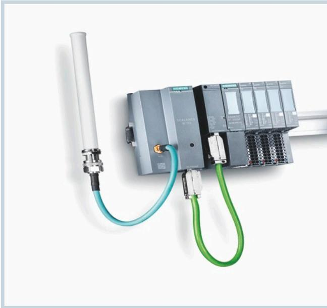
Space-saving and cost-effective setup of wireless network with SCALANCE W components, and seamless integration of the SIMATIC ET 200S into the industrial WLAN.
