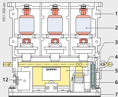
Construction of the 3TL8 vacuum contactor
