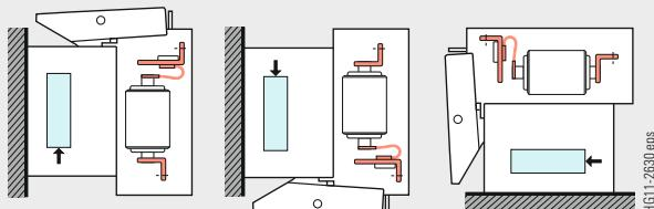
The arrow shows the arrangement of the terminal strip
