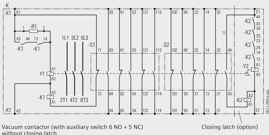
1) In 3TL6133 and 3TL6135 contactors (with withdrawable terminal strip), the current must be deactivated externally via the unlatching coil.
