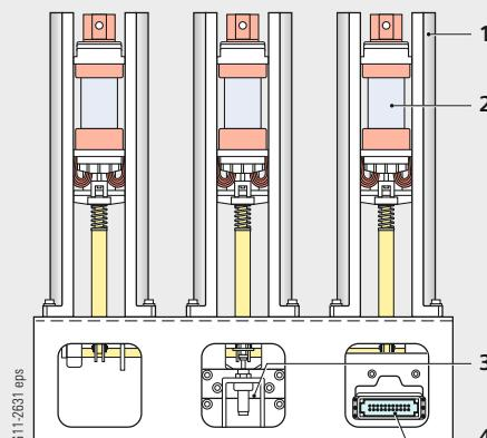
**Construction of the 3TL7 vacuum contactor**
