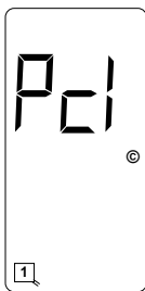
Loop Check Pending Indication
