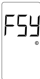
Parallel Synch Mode Failure Indication
