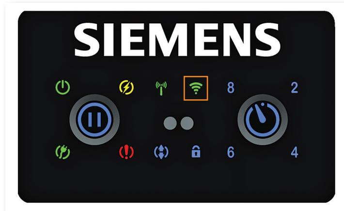
**STEP 4** Connect your web enabled device (computer/tablet) to the VersiCharge Access Point. To do this, find the available wireless networks which your computer or tablet can connect to and select the network starting with the letters 'VS' as pictured below. If you want to verify you are connecting to the correct VersiCharge network, make sure the serial number on the label at the top of your VersiCharge unit matches the network which your web enabled device is now connected to.
