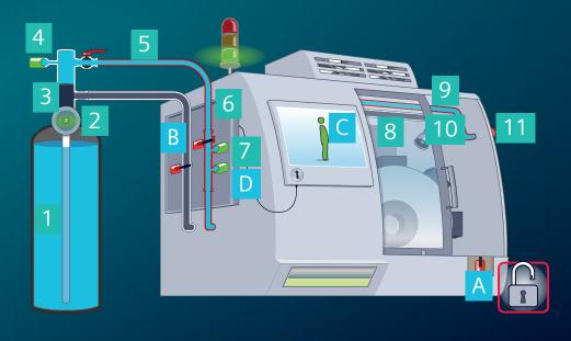
**Requirements for door release (personal protection):** The machine door can be opened **A** when the safety valves for extinguishing activation **B** are blocked, the machine operation **C** is blocked and extinguishing **D** was not activated.
