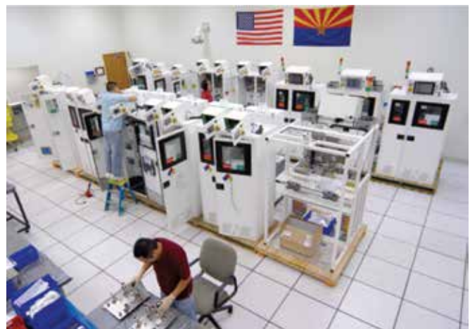
Gas cabinets being assembled in Norcimbus' 20,000 square foot facilities in Phoenix, Arizona. Norcimbus is a leader in developing and manufacturing innovative high quality UHP process gas systems and controls.
