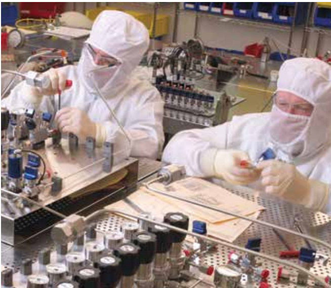
Norcimbus clean room technicians assemble high purity gas panels that come in a variety of manual, automated, or semi-automated formats.
