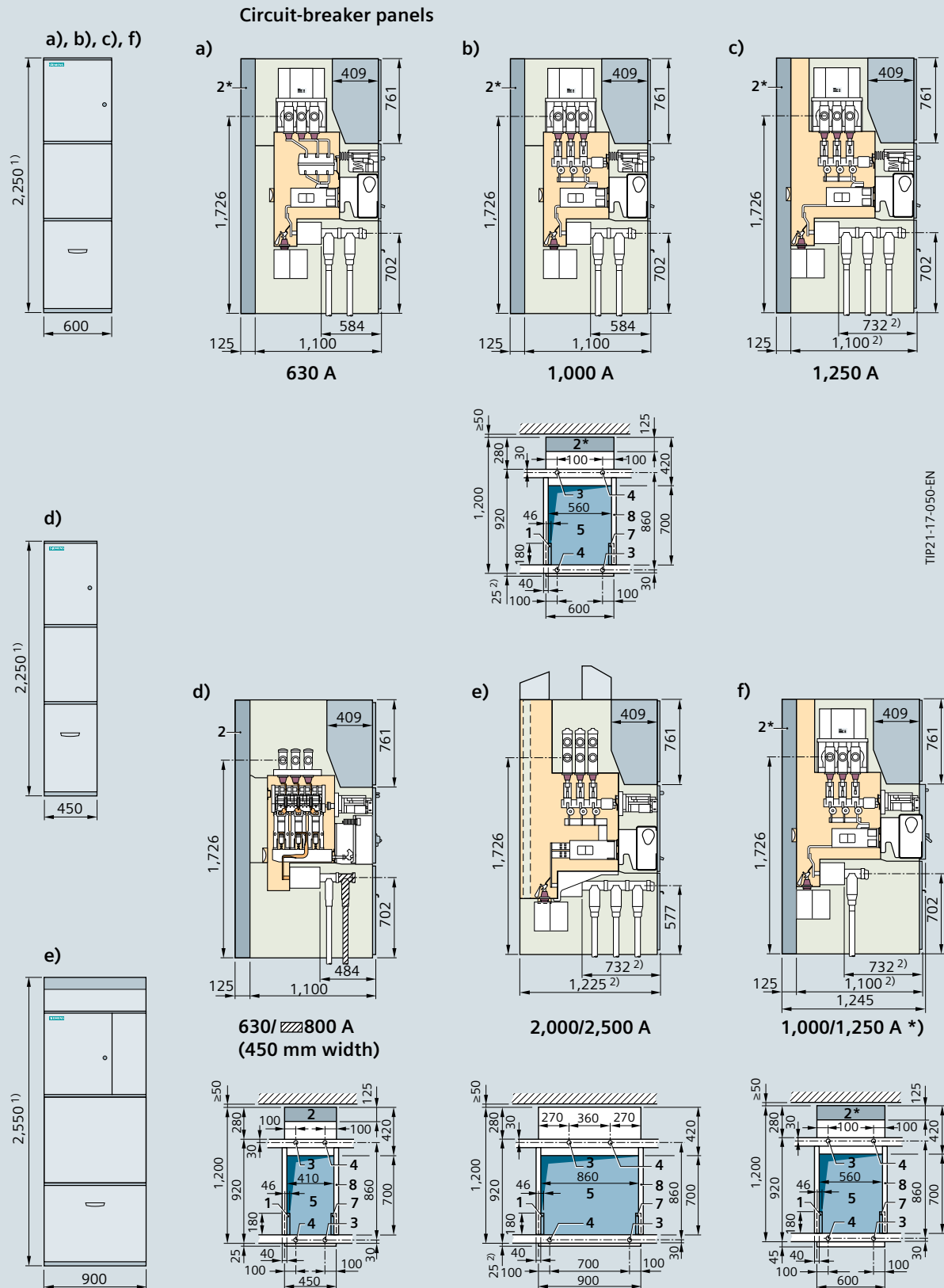
Fig. 3/4: Front and side views as well as mounting surfaces with floor fixing points for circuit-breaker panels with cable connection from below (dimensions in mm; legend and footnotes see Fig. 3/3 on page 54)
