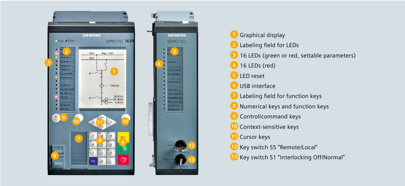
Fig. 8/7: SIPROTEC 5 operation panel: base module (left) and expansion module (right)
