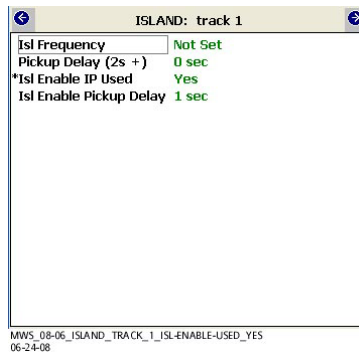
Figure 10-54: The ISLAND: track “N” “Isl Enable IP Used” Window
