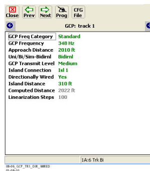
Figure 6-194: Setting the Directionally Wired Parameter
