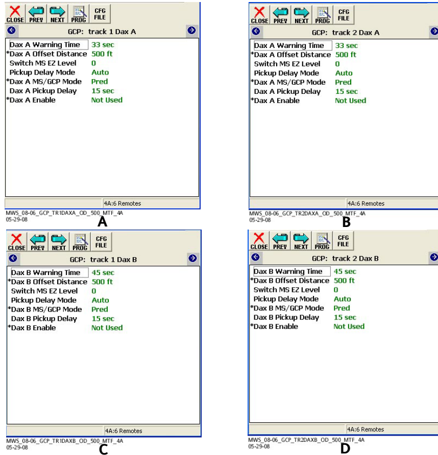
Figure 6-53: DAX Configuration For Remote Preemption Start
