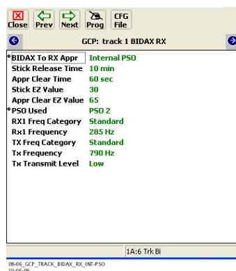
Figure 10-44: The GCP: track “n” BIDAX RX Window
