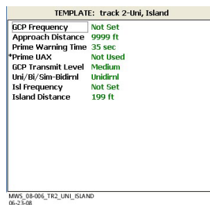
Figure 10-9: The TEMPLATE: track “N”-Uni, Island Window with Preemption set to Off and Prime UAX set to Off
