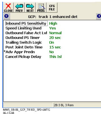
Figure 5-67: Track N ED Speed Limiting Used
