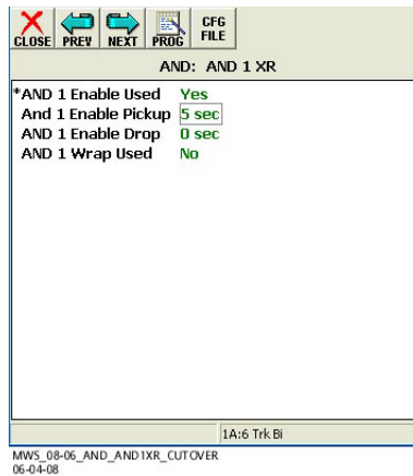
Figure 5-94: AND 1 XR Configuration During Cutover (Train Detection)
