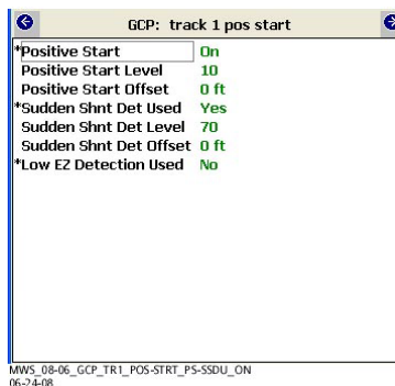
Figure 10-50: The GCP: track “N” pos start “Positive Start and Sudden Shunt Det On” Window
