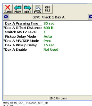
Figure 6-29: Pickup Delay Parameters For DAX With Non-Zero Offset Distance
