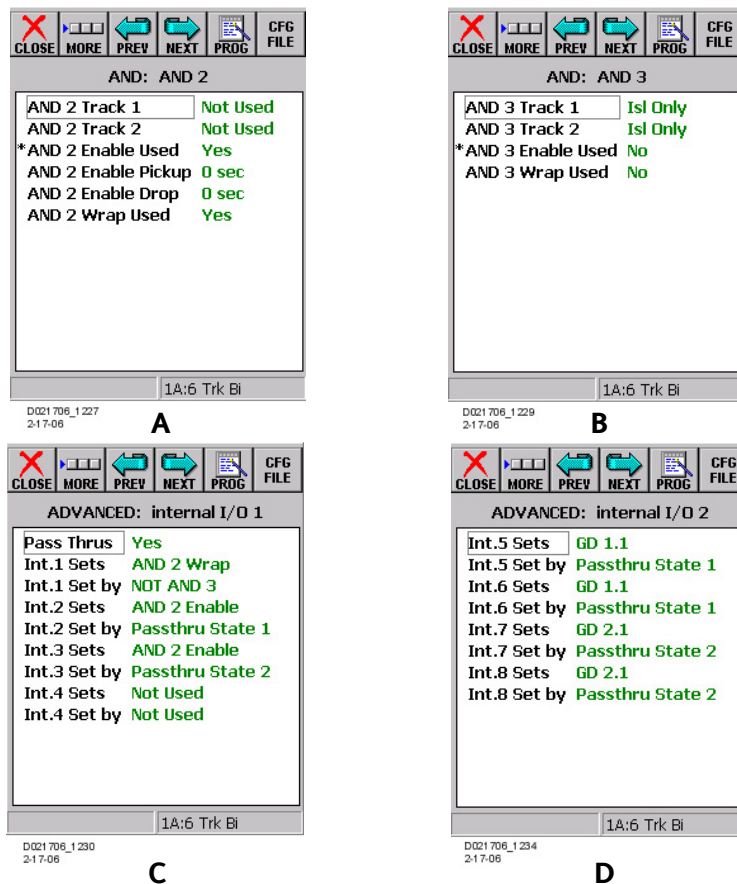
Figure 6-103: Internal I/O Example 2: AND Outputs
