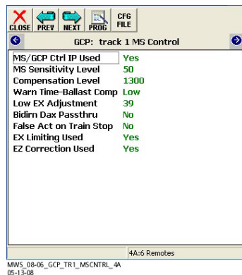
Figure 5-62: MS Sensitivity Level Parameter Adjustment Window
