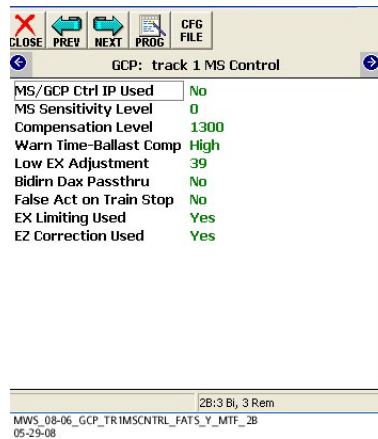
Figure 6-136: The Bidirectional DAX Passthru parameter
