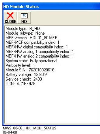
Figure 6-172: The HD/LINK Module Status Window
