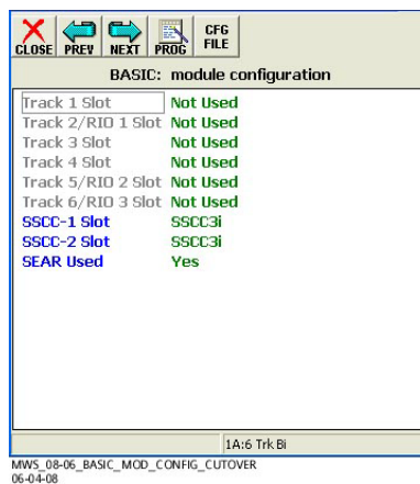
Figure 5-93: Basic Module Configuration During Cutover (Train Detection)
