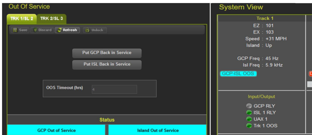
Figure 2-15 Island Out of Service Indications on WebUI
