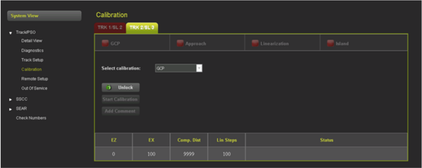
Figure 4-5 Track Calibration Screen
