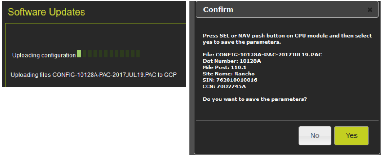
Figure 6-6 WebUI: Configuration Upload Progress and Final Check
